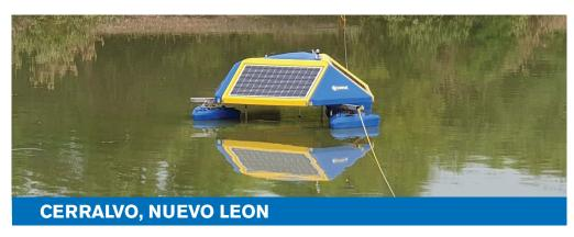
Installation in a non-aerated and organically over loaded pond (250 lbs BOD/ac/day). A multi-probe meter monitors dissolved-oxygen, pH, temperature and several nutrient values in real time. Nuevo Leon university is taking influent and effluent samples weekly to document performance.
