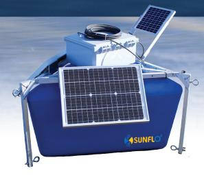
Self-contained, portable water quality sensors measuring and documenting treatment system conditions in real time in the middle of the pond.
